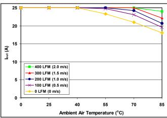
Figure 7: Maximum output power-derating curves vs. ambient air temperature for airflow rates of 0 LFM through 400 LFM with air flowing lengthwise from output to input (nominal input voltage).
