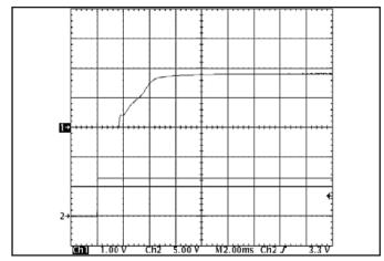
Figure 10: Turn-on transient at zero load (2 ms/div).
