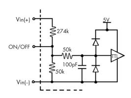
Figure B: Internal ON/OFF pin circuitry
