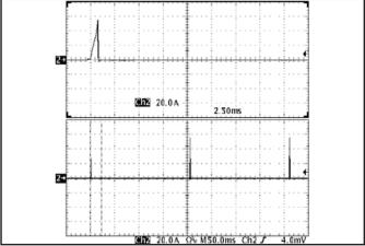
Figure 18: Load current (20A/div) as a function of time when the converter attempts to turn on into a 10 m $\Omega$ short circuit. Top trace (2.5ms/div) is an expansion of the on-time portion of the bottom trace.
