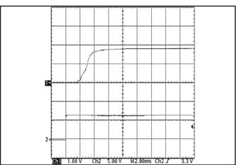
Figure 9: Turn-on transient at full load (resistive load) (2 ms/div).
